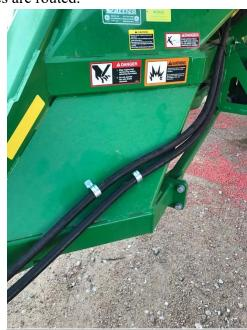
(above: not shown) Install protective hose-wraps to L of clamps to protect against stalk abrasion.
