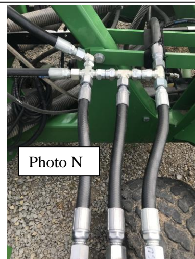
Photo M - Using 2 cartridges and accumulator. 'Equalizer' fittings joining the feeder hoses. Photo N - Using 3 cartridges (to supply higher numbers of openers) and accumulator. 3 short feeder hoses merge into the 2 long feeder hoses (one for each rank).
