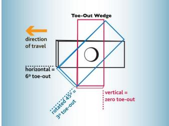
Remove closing wheel & spacers. Place wedge with wide end towards front of planter for the full 6° of toe-out (a suggested starting place for setup for soddy conditions or tough clay soils that resist closing, such as southern USA), or rotate the wedge by 45 degrees (see diagram) to reduce the toe-out to 3 degrees B a good starting place for mellower soils, such as in Canadian prairies. Install
