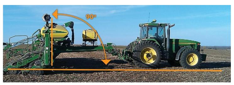
bolt the clevis or pull loop onto the planter tongue—move the loop or clevis to the lower holes to raise the planter nose.
