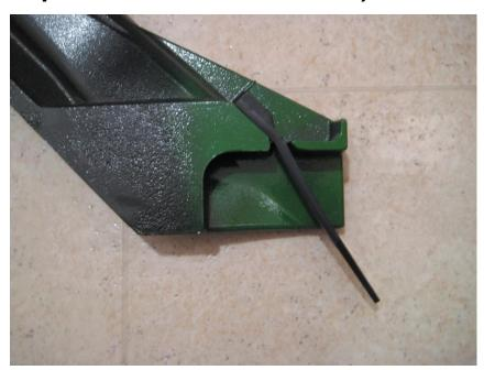
series, there can be enough rounding of the side of the slot where the flap installs that it pushes the flap over into the blade—if necessary, carefully grind notches in the upper end of the flap to get around this (see photo).
