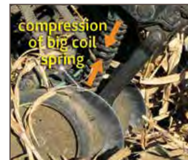
Inadequate down-pressure causes shallow furrows and more misplaced seeds. The only meaningful indicator of down-pressure is compression of the big coil spring.
