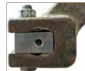
No need to replace worn depth adjustment arms with the new solid axle shaft.
