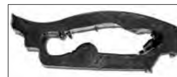
Cross-section of Exapta's PolyFlex tire: polyurethane with a hollow core, that can flex.
