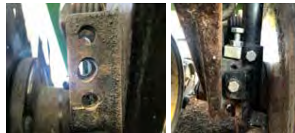
Far left: seed boot holes are 'egged' out, causing boot slop.
