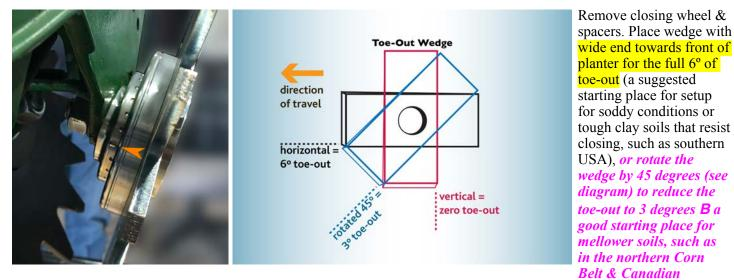
*prairies.* Install closing wheel using original spacers & bolt. Hold wedge in place while tightening bolt. The wedge won't turn after bolt is tightened. [Note on JD 1700-series: it may be wise to put a flat washer under the locknut on inside of closing bracket, to help distribute the load since bolt is now at an angle and the cast material is slightly brittle.]
