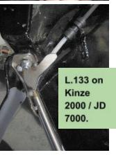
**4)** If applicable, reinstall front screw in Keeton Universal bracket (*the bracket's wedge gets discarded*; the bracket is just fine without it). Install zip-tie around 1/4" line and hole in Valion. Use a double-wrap of the zip-tie.
