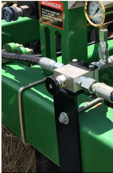
Photo K. UniForce valve block on box drill. Yours should have a 90-degree fitting on outboard side to reduce loop of hose needed.
