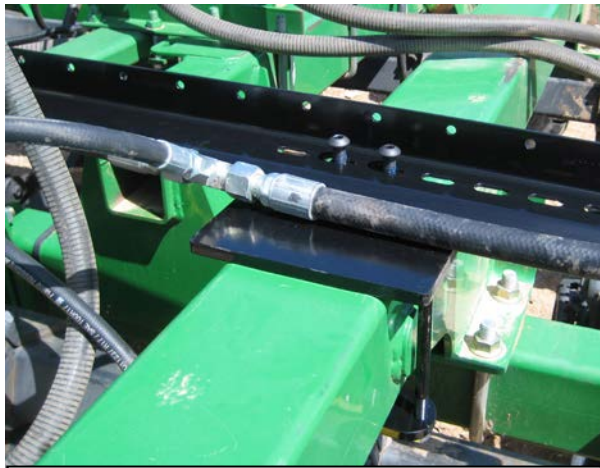
Photo G. RH wing: rear tray, outer end. Brkt #0003. Button-head bolts need to be tightened yet. Header hose is already assembled & lying across the U-bracket here.
