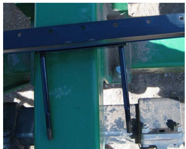
Photo E. RH wing: front, outer end. Brkt #0004. Tray is attached via ½ x ¾" buttonhead bolts threaded into U-bracket. Assembly pulled up off the frame tube for viewing.
