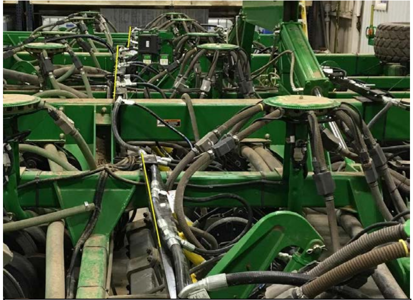
Photo B. Yellow lines show the offset of tray position on center vs wings. This is an 1895, hence the extra towers and extra rank. All trays go on top of frame tubes except center rear on CCSs.
