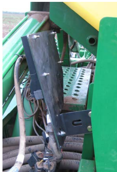
Photo H. When rear rank gets UniForce, the electrical bracket must be replaced w/ Exapta's #0023 (shown).
