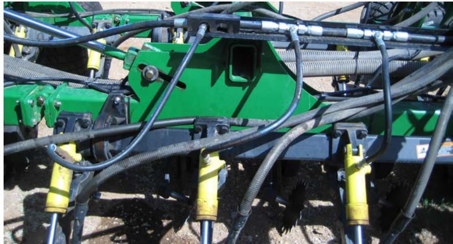
Photo M. 'Bridge' hose between drill sections in upper-left of pic.
