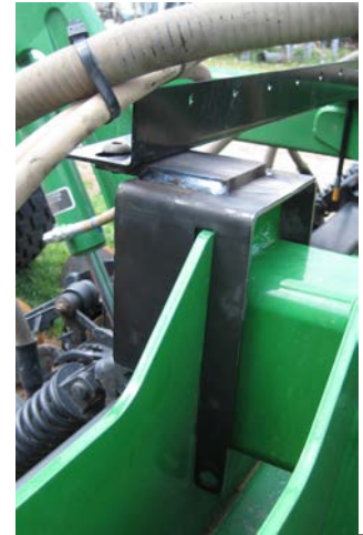
Photo F. LH wing: rear tray, inner end. Brkt #0006. Thru-bolt not yet installed here.
