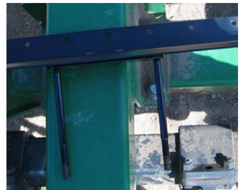
Photo E. RH wing: front, outer end. Brkt #0004 on this 1890. Tray is attached via 1/2 x 3/4" buttonhead bolts threaded into U-bracket. Assembly pulled up off the frame tube for viewing.
