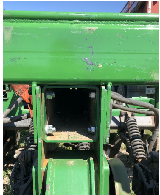
Spacer plate installed on RH side. Not all drills need this (depends on tube dimensions that JD used).
