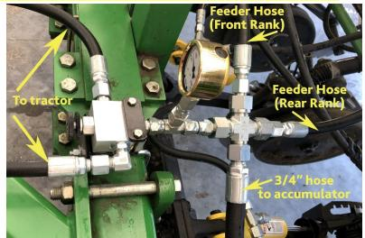
3) Route the 165" hoses along the tongue, and secure with large zip-ties. Install the high-flow (5/8" body) quick-couplers (provided) and adaptors on the tractor end of the hoses. Tighten fittings.
