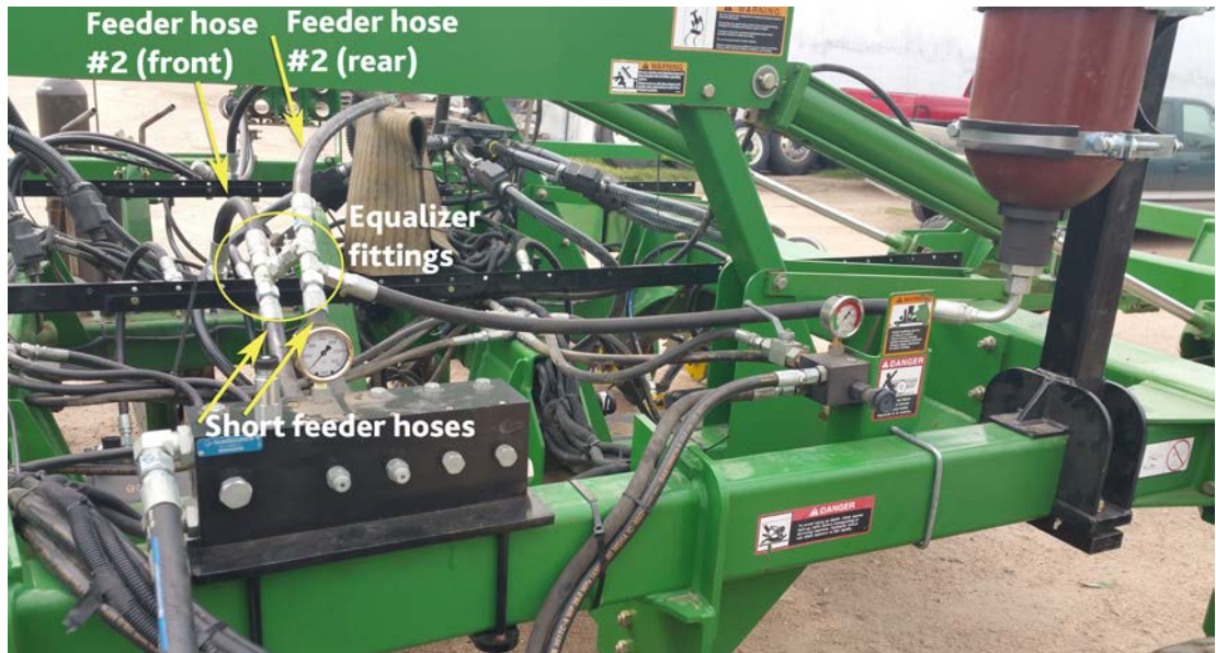
Photo N. 'Equalizer' fittings joining the feeder hoses on an 1890 w/ air cart. If 3 cartridges were used (to supply higher numbers of openers), there would be 3 short feeder hoses which would merge into the 2 long feeder hoses (one for each rank).
