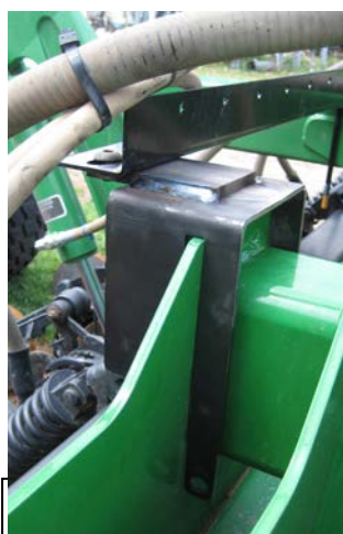
rear tray, inner end on 1890. Brkt #0006. Thru-bolt not yet installed. (1895's #0013 is slightly different)
