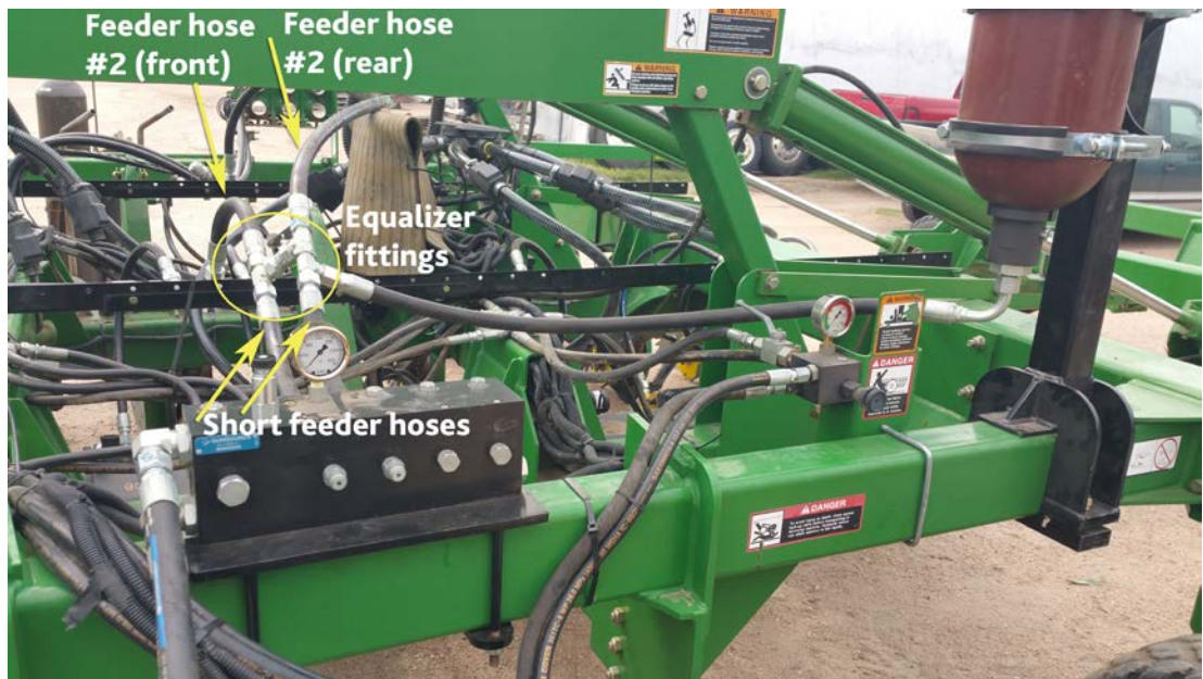
Photo N. 'Equalizer' fittings joining the feeder hoses on an 1890 w/ air cart. If 3 cartridges were used (to supply higher numbers of openers), there would be 3 short feeder hoses which would merge into the 2 long feeder hoses (one for each rank).
