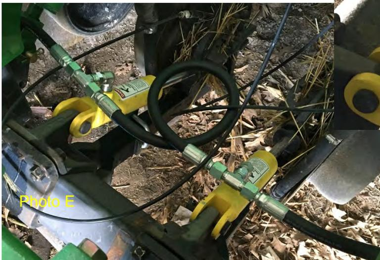
longer hoses to span where the rockshaft's supports & torque cylinders are, and some 90s to help with this (see schematic & Photo D). Also install one T-fitting (M-M-F) in the middle for 'feeder' hose (1/2") coming from the UniForce manifold/valve block.
