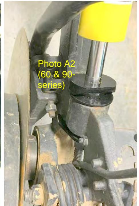
4) Set cylinder + bushing into large flat washer, then into hole in cast opener (see photos A1, A2).
