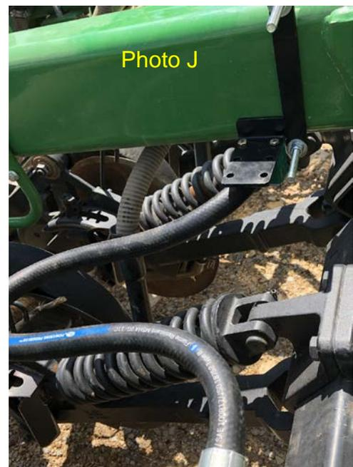
5) Install the 'bridge' hoses at the hinge points for the wings—these are  $\frac{3}{4}$ " hoses (of lengths indicated in schematic) that join the header hoses. Bridge hoses go *below* the frame when joining the *rear* inner & outer wings. Tighten all fittings. Tether the hoses so they stay away from pinch points at the hinges (see Photos H, J—in Photo J, the bridge hose makes a big loop: no tethering is
