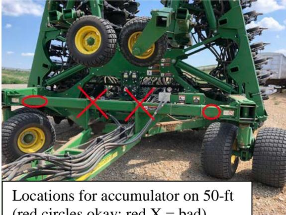
5) If an accumulator is being used: assemble it, mount it on the frame (see photos), and connect it to the fittings that equalize the feeder hoses just behind the valve block (*don't use the port on the valve block*). The accumulator should arrive pre-charged, unless the system was shipped by air. Pre-charge on accumulator should be 400 psi. Tighten all fittings.
