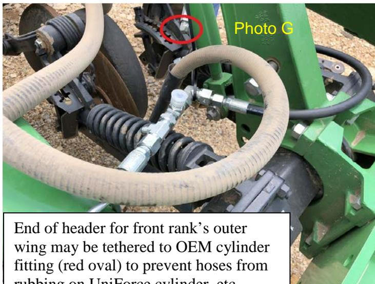
End of header for front rank's outer wing may be tethered to OEM cylinder fitting (red oval) to prevent hoses from rubbing on UniForce cylinder, etc.
