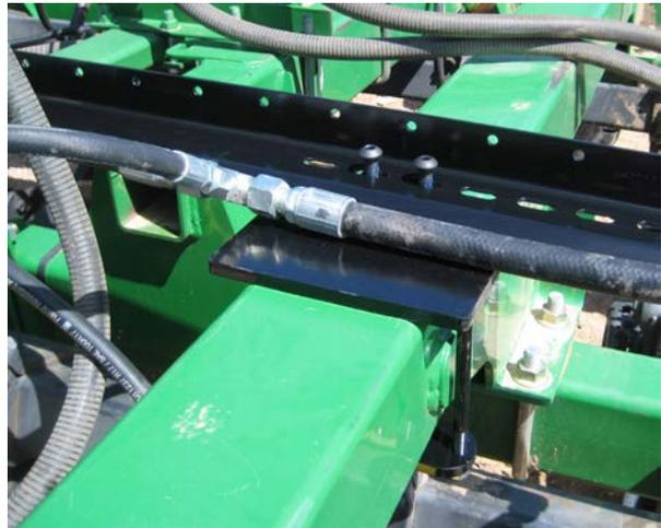
**Photo G. RH wing: rear tray, outer end (40' 1890). Brkt #0003. Button-head bolts need to be tightened yet. Header hose is already assembled & lying across the bracket here. 1895 uses a narrower bracket at this location.**
