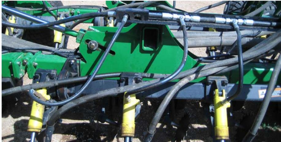
**Photo M. 'Bridge' hose between drill sections in upper-left of pic.**
