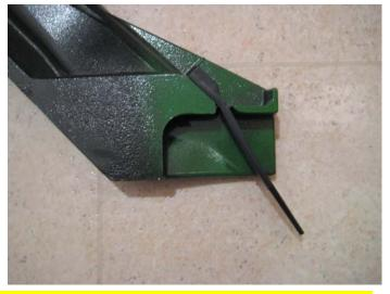
installs to prevent the flap from staying away from the blade—if necessary, carefully grind notches in the upper end of the flap to get around this.
