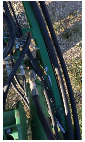
3) If hitch is equipped with hydraulic weight transfer, secure the hoses away from the cylinder or they'll get pinched, as has happened in the photo.
