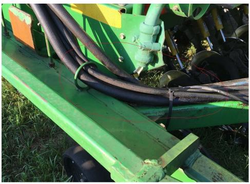
2) Cut off ~2" of pipe handle, or else it will gouge into the hoses.
