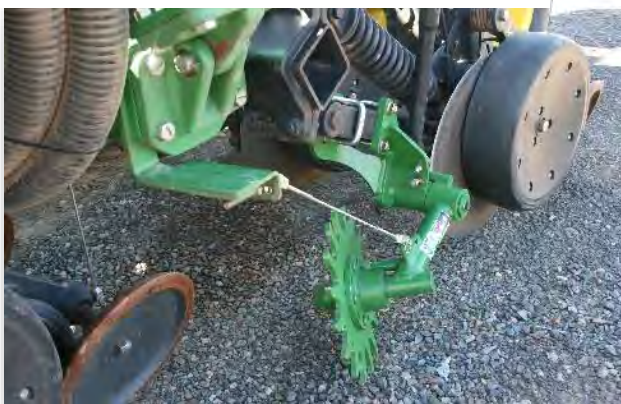
Installed Aricks Wheel left hand side. Note the position of the 'L' bracket at left of photo.
