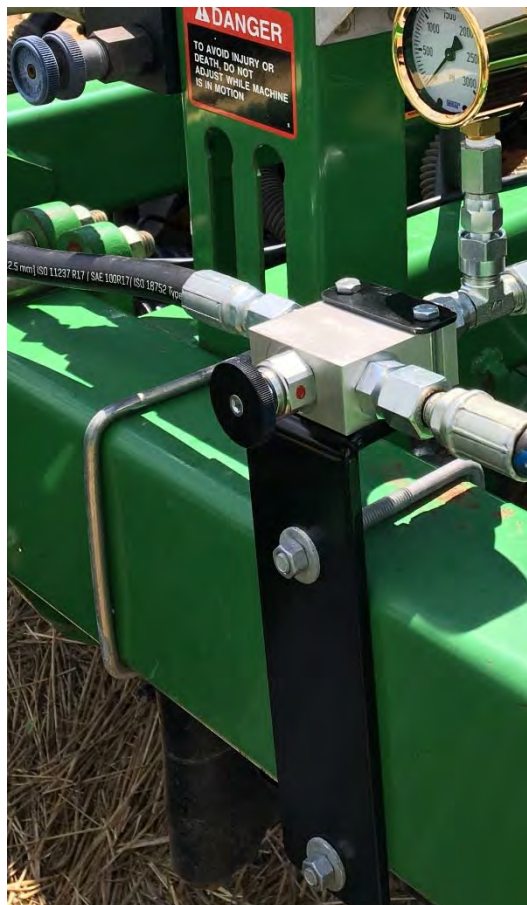
Photo K. Line-body valve block installed on box drill. Yours should have a 90-degree fitting on the outboard side to reduce the loop of hose needed.
