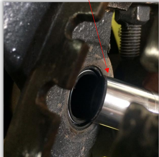
Chamfered end inserted first
