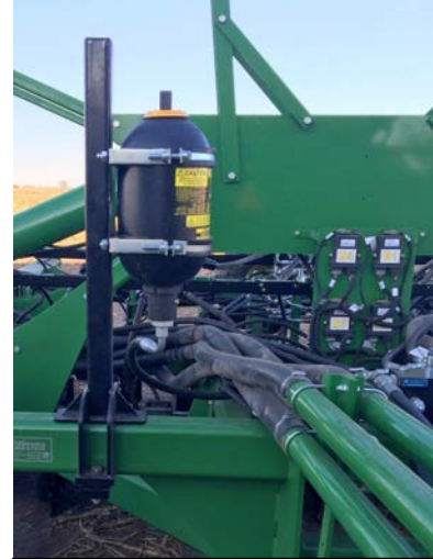
Accumulator on 60-ft w/ TBT cart. Note: 50-ft may have clearance issues with dolly wheels when folded with an accumulator in this location.
