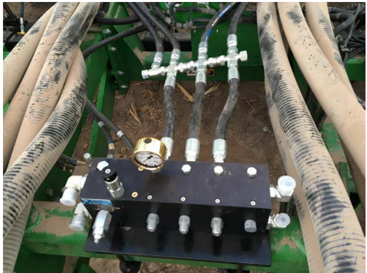
Photo M. On a 5-section drill with TBT cart. 3 cartridges used, going into 4 long 222" feeder hoses, with places for 2 accumulators to plumb in on both ends of equalizer fittings.
