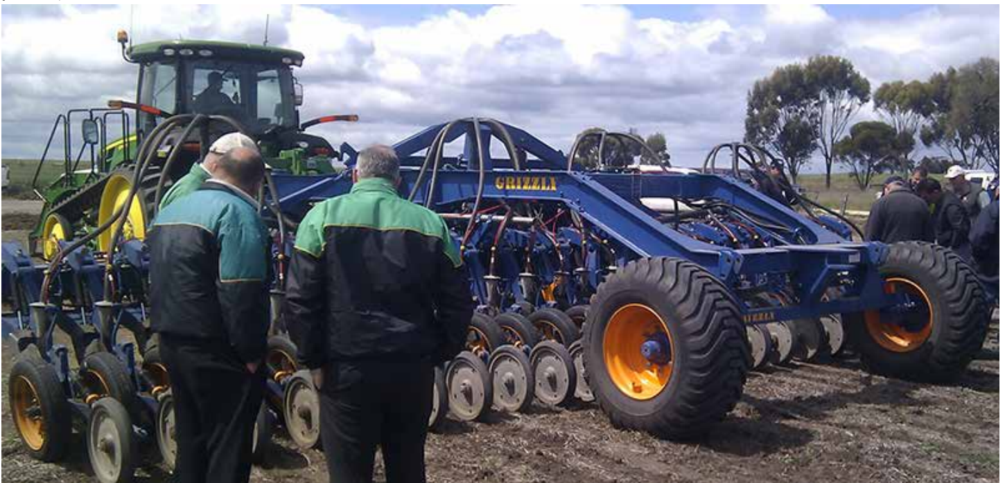
Australian-built air drill. Note how high the risers are and the steepness and straightness of the secondaries all of which is very desirable for uniform flow to each row. Note also the diffusers in each secondary, just above the opener. The drill's owner Robert 'Ruwy' Ruwold also runs SeedVUs in each head.
