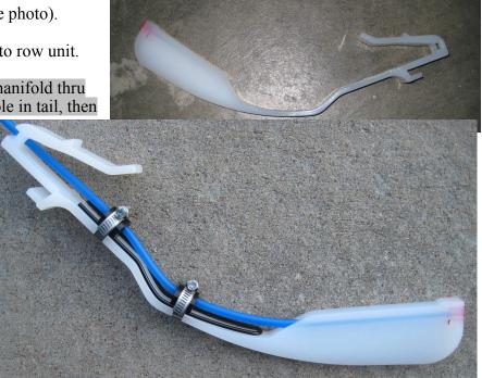
Blue tubing used here for visibility. Customers are strongly encouraged to use thick-wall black tubing instead, for durability.
