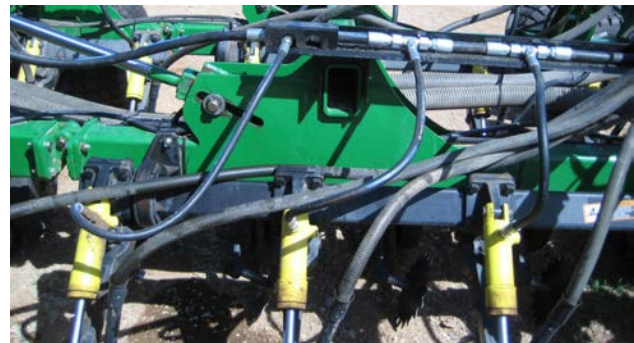
Photo M. Note the 'bridge' hose between drill sections in upper-left of pic.
