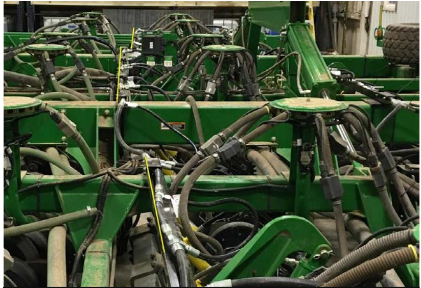
Photo B. Yellow lines show the offset of tray position on center vs wings. This is an 1895, hence the extra towers and extra rank. All trays go on top the framework, except on CCS models where the center-rear is under the frame.
