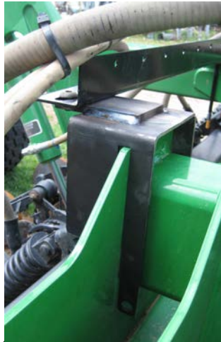
Photo F. LH wing, rear tray, inner end on 1890. Thru-bolt not yet installed here.
