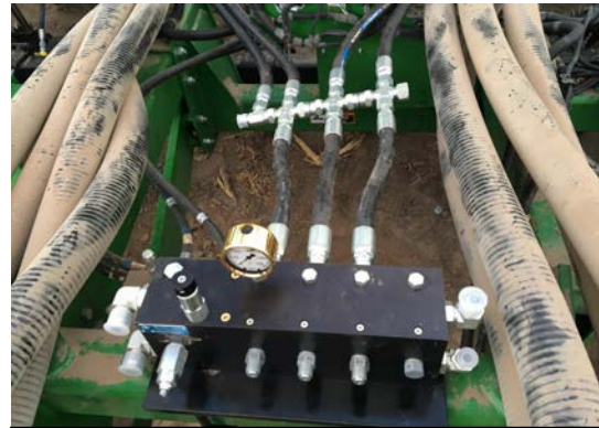
Photo N. 'Equalizer' fittings joining the feeder hoses. Photo shows a 60-ft with 72 openers, so 3 cartridges merge into 4 feeder hoses going out to the headers, whereas on 3-section drills, only 2 feeders go to the headers.
