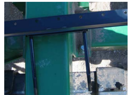
Photo E. RH wing, front, outer end (on 40-ft drill). Tray attached via ½ x ½" buttonhead bolts threaded into U-bracket. Assembly pulled up off the frame tube for viewing. The center section's trays attach the same way.
