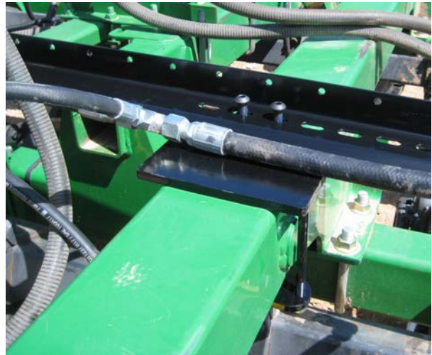
Photo G. RH wing, rear tray, outer end (40' 1890). Button-head bolts need to be tightened yet. Header hose is already installed & lying across the U-bracket here. 1895 is slightly different at this location.
