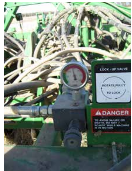
On the JD 50/60/90-series NT drills, in tough soil conditions such as the southern half of USA, hydraulic down-pressure often needs to be set well into the red. But extra frame weight is required!
