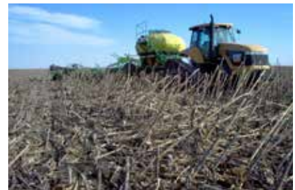
Another drill running in the very mellow soils of the eastern Dakotas. No weight on wings except the markers. It is sufficient, since down-pressure requirements are not extreme. Note that the wing isn't lifting (compare to horizon & center section of drill).
