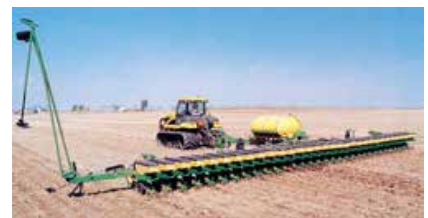
Carrying all the weight on the center section poses problems. Here, we can see that the center rows are furrowing deeper (more row cleaner action) due to the weight. This is where active down-force systems become valuable, such as Precision Planting’s AirForce.
