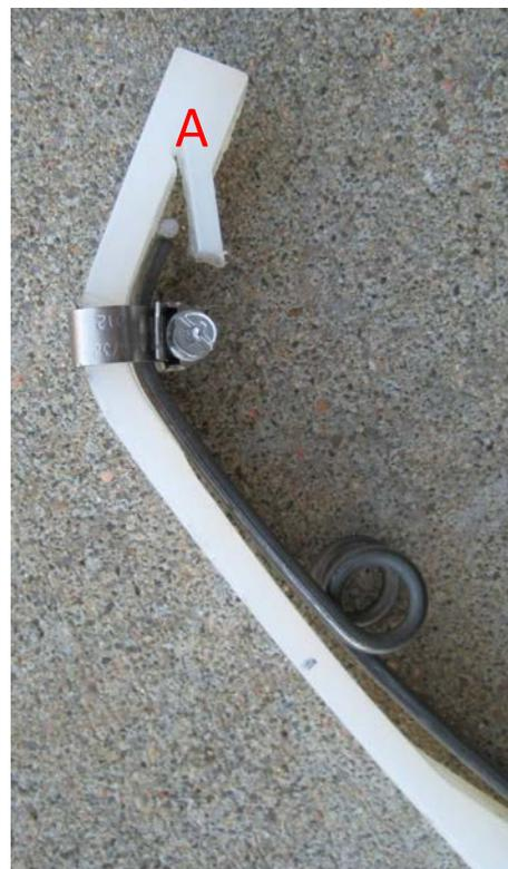
2) Position steel tab on Mojo Wire as shown in Photo B, as far rearward as it will go. Mark the hole location and drill a 3/16" hole **that is at 90-degrees to the plane of the upper Keeton tail surface below it (see photo C).** Ream hole very slightly.
