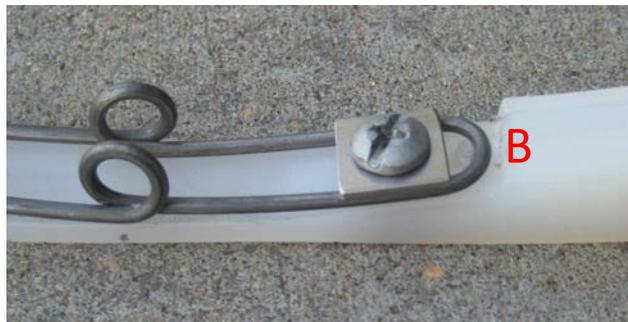
3) Insert screw thru tab and tighten (Photo B).
