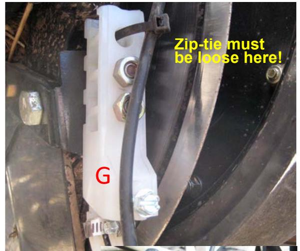
iv) If using the liquid feature: Attach tubing to uppermost hole in plastic receiver with a zip-tie to keep it from rubbing on the blade, but *leave the zip-tie as loose as possible (see Photo G) so that tubing doesn’t kink when tail flexes to maximum. Then zip-tie farther up the opener but as loose as possible (see Photo H, towards bottom of pic).* Finally, secure tubing farther forward (for instance, front of depth-adjust notches) and these should be zipped tight.
