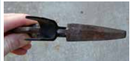
A severely worn OEM seed tube guard. Note that the sides have worn in an arc due to blade flex.
