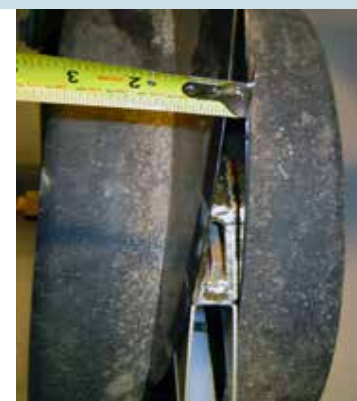
The furrow will have a flat bottom if blade flex is minimized. Seed depth is much more consistent if blade flex is minimized.
