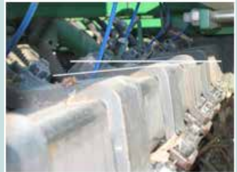
Rockshaft should slope rearward, as shown by the white lines. (Drill is traveling towards the right.)
