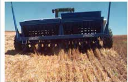
AVEC drill at Dakota Lakes Research Farm. It is built in Argentina and has a very functional opener design as well as a unique rapid-response down-pressure system that keeps equal pressure on all openers at all times. At least one manufacturer in Europe is working to integrate these features into a robust opener on an air seeder frame. Hopefully they'll get it right, and eventually introduce it to North America.
