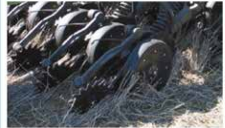
Deere 90-series drill opener. Many no-till drills now have features to make them more precise, i.e., like a planter, such as using depth-gauge wheels alongside the opener blade. This drill model has some attributes that surpass OEM planters, such as an in-furrow firming wheel completely separate from the closing wheel. However, this model still cannot equal a well-tuned planter for placement.
