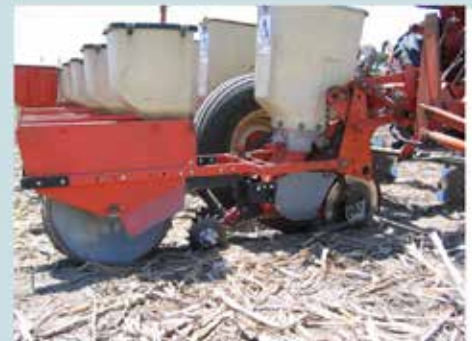
In the 1960s, planter openers gauged their depth from trailing treader wheels. Essentially all manufacturers have now gone to depth-gauging wheels alongside the opener blades, for greater precision.
