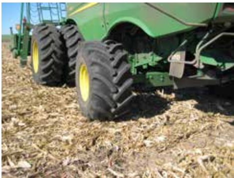
Michelin Mega X Bib 750/65R26 on the back of an S680 combine. It's possible to go to 850s (which are Deere-approved), although I hear of tie-rods breaking occasionally.
