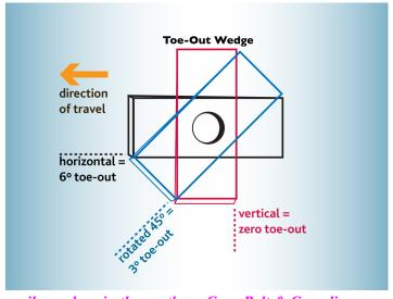
the toe-out to 3 degrees – a good starting place for mellower soils, such as in the northern Corn Belt & Canadian prairies. Install closing wheel using original spacers & bolt. Hold wedge in place while tightening bolt. The wedge won't turn after bolt is tightened. [Note on JD 1700-series: it may be desirable to place a flat washer under the locknut on inside of closing bracket, to help distribute the load since bolt is now at an angle and the cast material is slightly brittle.]
