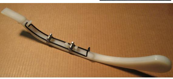
range of the tensioning screw: 3/4-turn may cause a 1 lb change in pressure. In the field, you should adjust (tighten) this screw further, but starting with too much pressure can damage Keeton bracket.
