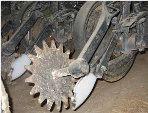
The Fin moves independently of the opener, and has nearly continuous pressure.
