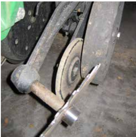
Deere 60/90-series. This is also a seed-lock wheel, but larger diameter— 9 or 10 inches, depending on manufacturer.
