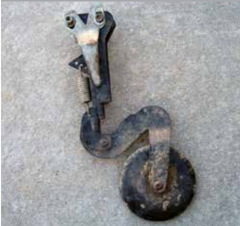
Small seed-lock wheels for planters were all the rage in the mid- and late-'90s, but quickly fell out of favor due to mud accumulation problems—most of which was due to the axle being down too close to the mud, and the arm too close to the wheel.
