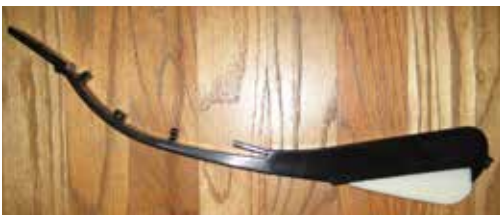
The Flo-Rite seed firmer, introduced in 2014, with Beck's Hybrids being the exclusive distributor. These have about 60% more pressure than a Keeton when new, which is wonderful! However, they still need Mojo Wires for all except the mellowest of soil conditions. Limited farmer testing in 2013 indicates they wear only half as fast as Keetons, plus the lower end is replaceable on the Flo-Rites. What is unknown is how well they shed mud in sticky clays, a.k.a. gumbo.
