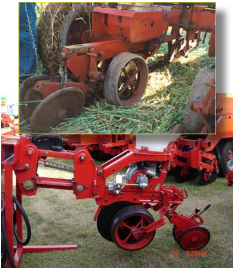
Almost all planters worldwide have had gauge wheels alongside the blades for many decades. Brazilian models old & new (2005) shown here.
