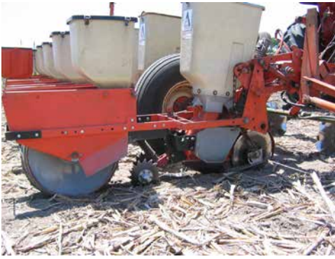
A relic from the past, when planters gauged depth from trailing packer / treader wheels. Despite being one of the earliest planters halfway capable of no-till seeding, the results were pathetic with 50 – 60% emergence, and no consistency in timing of emergence. This one has been modified with serrated furrow-covering discs and sliding 'heave-limiters' alongside the opener blades.
