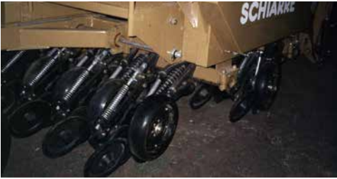
Clones of the John Deere 50/60/90-series gauge-wheel drill openers in Russia & Argentina.
