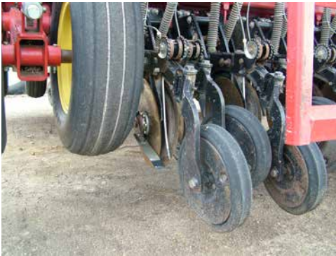
Press-wheel drills have replaced the hoe or knife with rotating disc blades to create the furrow, but still gauge their depth from the trailing packer or press wheel.
