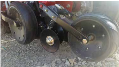
Case-IH Early Riser planter opener. Covering discs are suspended from arm that holds the treader wheel (which is capable of going to zero pressure).
