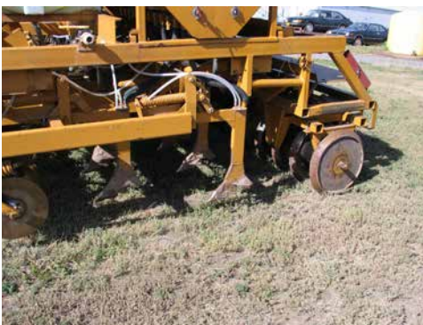
Hoe-drill from USA. Many shank/tyne openers, including air drills, are barely more sophisticated than planting sticks from a functional standpoint.
