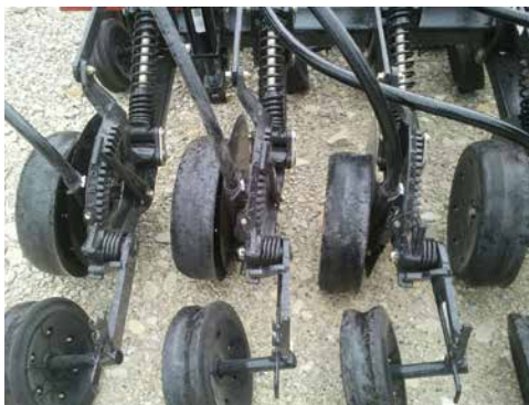
Case-IH P-500 / NH 2080 drill. The lack of an in-furrow seed firming mechanism is a big mistake for no-till (nor does the closing wheel do much in NT).
