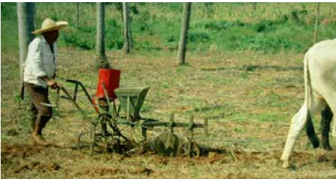
Although primitive by our standards, this seeder is depth-limited by an average of the wheel way out in front and the trailing wheel alongside the row (not over the row). The furrow was partly created by a separate implement. Note that this seeder also has a fertilizer hopper. Other than limiting depth entirely with a gauge wheel exactly alongside the blade(s), this sensing of terrain both ahead of and behind the blade is the only other configuration that makes sense for obtaining the best preciseness of depth (here, it's like a motor grader in that the blade forming the furrow is equidistant between the front & rear wheels sensing the terrain; completely unlike the Borgault 3710 and Morris-Razr designs described in the main text).
