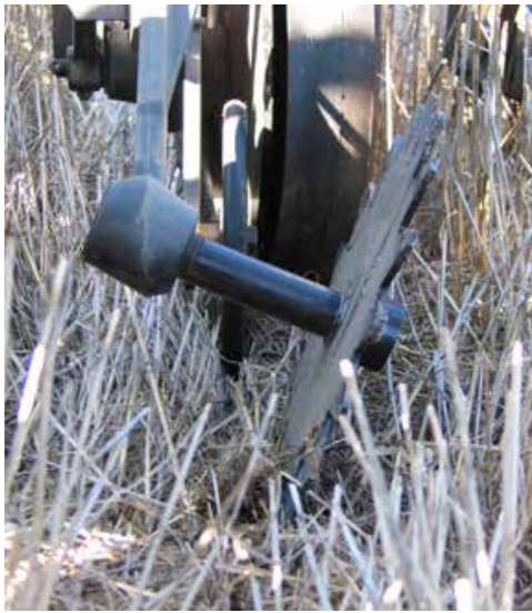
JD 90-series drill opener with aftermarket closing wheel to positively engage & crumble the sidewall. Only because depth-gauging & seed firming are already accomplished does it allow crumbler-style closing wheels
