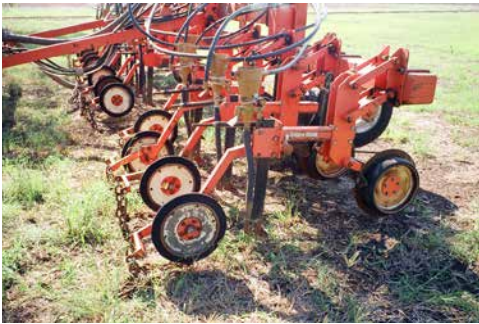
Light-weight shank opener in Australia with parallel-link and cutting coulter.
