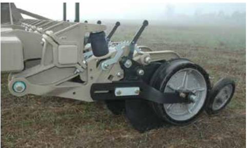
Another gauge-wheel drill design, by NDF of Australia. Note that the gauge wheel can be slid fore/aft, and the down-force is created by an air bag and not a spring. Nice. While still a swing-arm (radial) linkage, it is better than Deere's by the arm's flatter angle during operation. Still no method for in-furrow seed firming, however.
