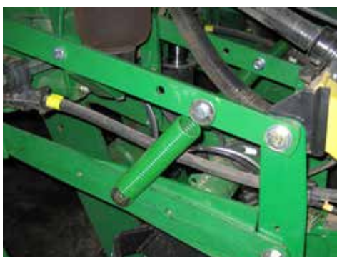
A different JD planter equipped with helper springs.
