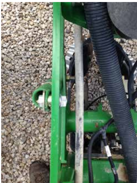
There's room for another pair of springs in-between the parallel arms on most of the Deere XP units with air bags. Adding 4 of the springs per row provides another 180 lbs of down-force, which is often quite a benefit in some geographies (or if unit-mounted fertilizer openers are used).
