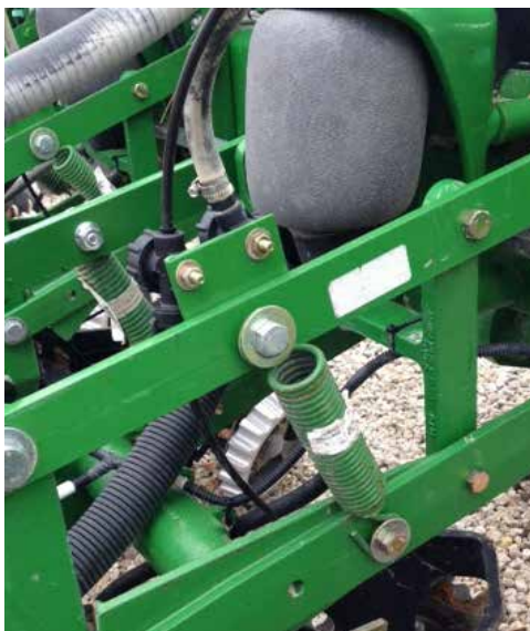
Air bags often need help. Two springs added here for another 90 lbs of down-force. There's actually a JD part # mentioned in the Owner's Manual for this improvement(!).
