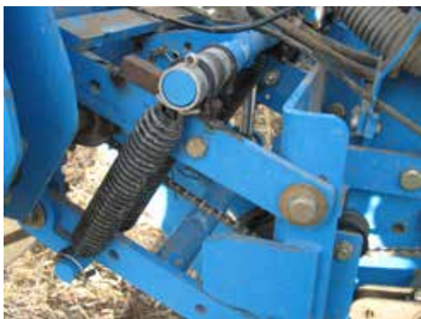
Monosem NG+4 can't develop anywhere near enough down-force for moderately firm never-till conditions without this additional preload from the ¾-inch block welded onto the link.
