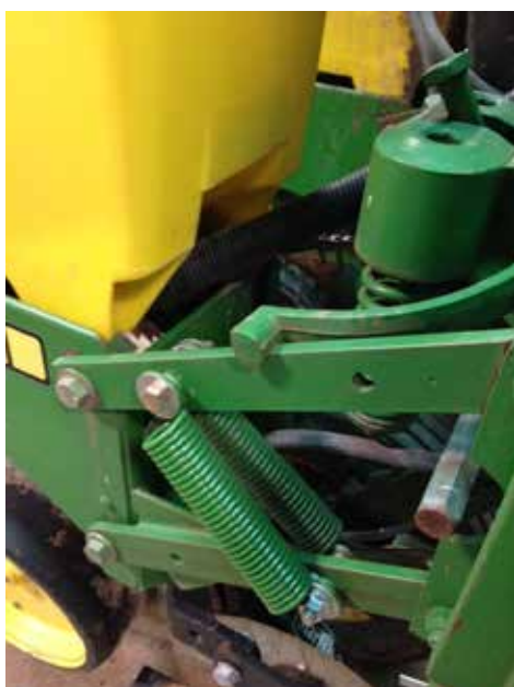
Sometimes the heavy-duty mechanical springs need the helper springs, too.
