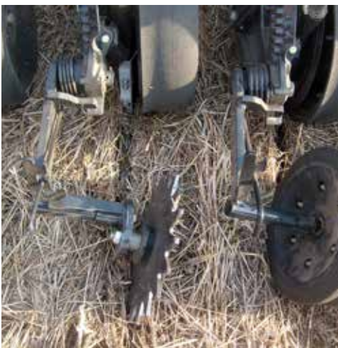
Exapta's closing bracket kit creates 7-degree toe-out to the direction of travel.
