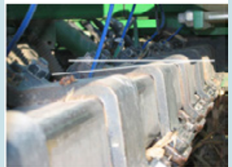
Rockshaft should slope rearward, as shown by the white lines. (Drill is traveling towards the right.)
